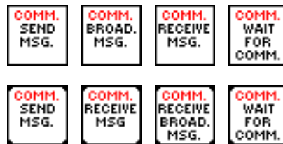
Figure 5.23: Send and receive VIs.
